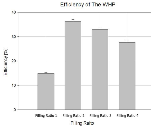
Figure 11. Efficiency of the WHP at different filling ratios
