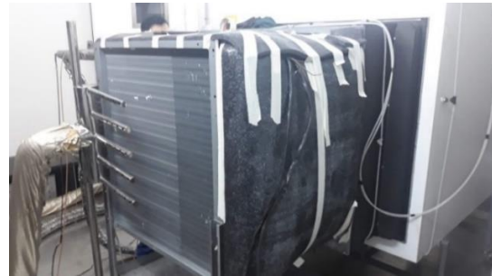
Figure 6. View of the insulated adiabatic region
