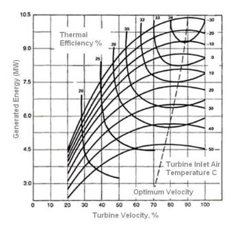
Figure:3 Performance Characteristics Depending on Combustion Turbine Inlet Air Temperature
