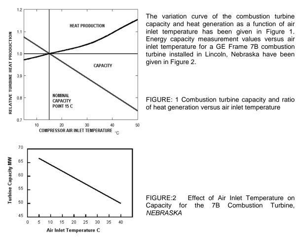
The combustion turbine capacities have been given for the +15°C temperature, 60% relative humidity and sea level as specified by ISO. Connection factors for capacities under other conditions must be obtained from the manufacturer firm. However, the following factors may me used for a general approach.
