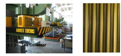
Fin Press Lines and fins processes according to mould, form and spacing. Tight contact achieved between tubes with the Arrangement and Blowing process. Main finned block
