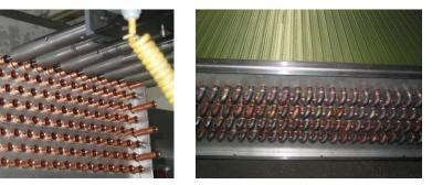
Figure: 7.2-3 View of the Tube Blowing Machine, the Blowing Process for Copper Tubes and of the Curves
