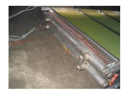
Figure:9.1 and Figure: 9.2 The Collector Processing Machine and Stainless Inlet-Outlet Collectors
