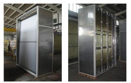
Figure: 13.1-2-3 View of the Cooling Unit Cell from the Drop Eliminator and the Filter sides (Filter cartridges are installed on location).
