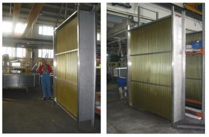
Figure: 6.1 Figure: 6.2 A view from the manufacturing process of the combustion turbine inlet air cooling coil.
