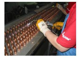
All copper tube-curve, copper tube-collector connections, connections used in frames and all connections of fittings should be done with the "Brazing" method and the solder wires used for soldering should be silver alloy solder wires.
