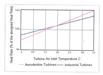
An increase in air inlet temperature of  $15^{\circ}$ C to  $38^{\circ}$ C increases the heat ratio. This leads to an approximate 4% drop in fuel efficiency. The drop in fuel efficiency can be prevented by cooling the combustion turbine inlet air. For a typical gas combustion turbine, cooling the inlet air from  $15^{\circ}$ C to  $6^{\circ}$ C lowers the heat ratio and increases fuel efficiency by approximately 2%.
